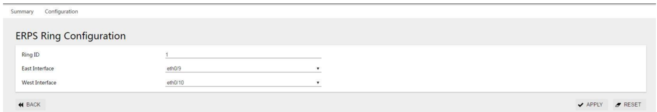
Figure 3-28 ERPS ring configuration interface
