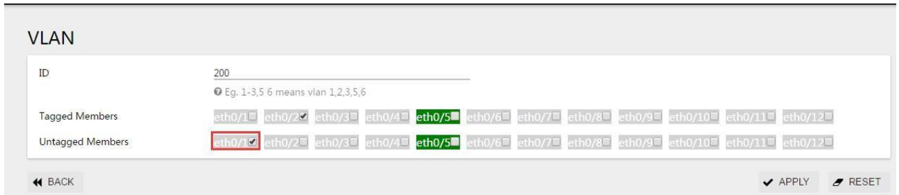
Figure 3-142 Configure Tagged and Untagged Member Ports
